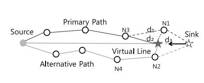
Fig. 3. Case that the Sink is Close to the Source
