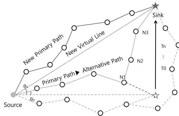
Fig. 5. The Multiple Hops Movement-Based Global Multipath Reconfiguration
