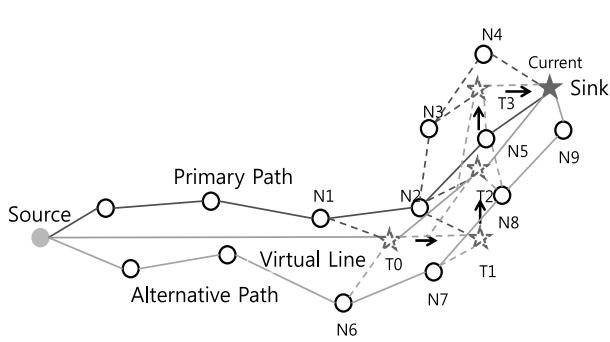
Fig. 4. The Multiple Hops Movement-Based Local Multipath Reconfiguration
