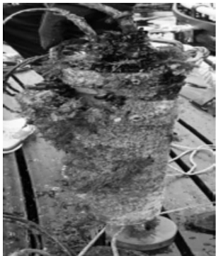
Fig. 2. Damaged Underwater Sensor by fouling[11]
