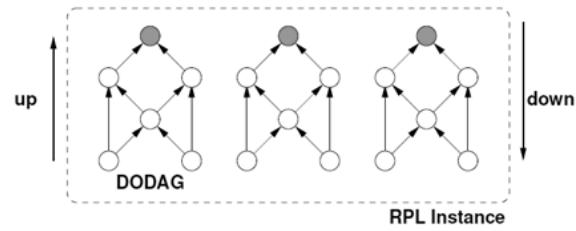
Fig. 2, RPL object and destination based DODAGs:
