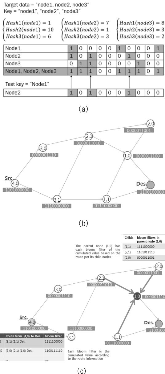
Fig. 6. (a) Bloom filter based light-weight IPv6 address,
