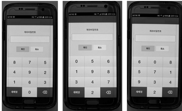
Fig. 2. PIN Entry Using the Randomly Placed Numeric Keypad
