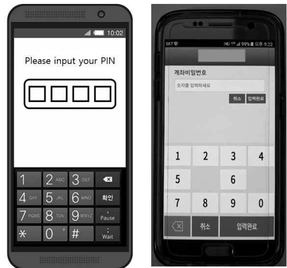
Fig. 1. PIN Entry Using the Normal Numeric Keypad, and PIN Entry Using the Numeric and Blank Keypad
