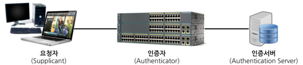
Fig. 1. Physical Elements of 802.1X
