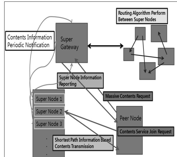
Fig. 2. Super Node &amp; Peer Node Structure
