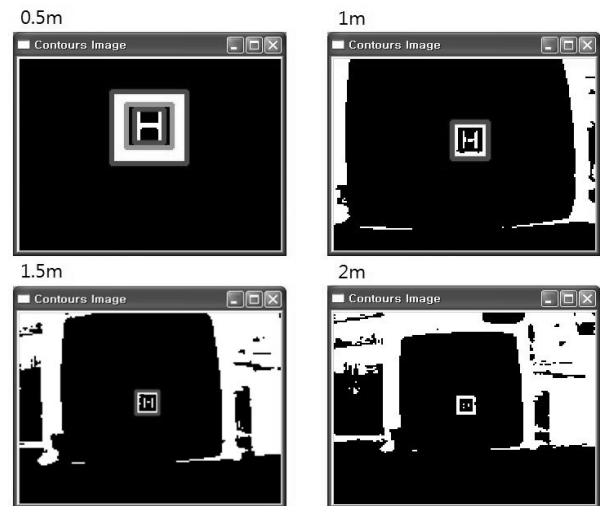
Fig. 14. The marker image displayed on the mock-up AGV with respect to the relative distance from the mock-up AGV to the marker
