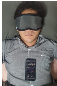
Fig. 12. Eye Patch-type Bio-signal Measuring Device Signal Measurement on a Mobile Device
