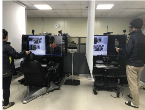
Fig. 7. Experimental Environment. Each Client Captures and Sends Video, Audio, and Haptics Data to the Other Client
