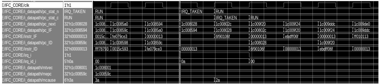
Fig. 5. Modelsim Simulation Screen. It Shows the Flow of PC and Instructions of Interrupt Handling
