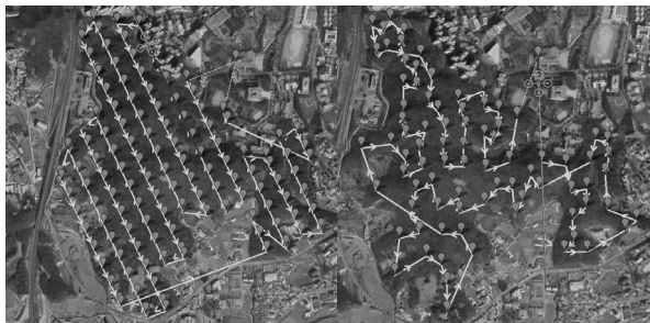
Fig. 7. (Left) Flight path of Drone with grid Method (Right) Flight Path of Drone with the Proposed Algorithm
